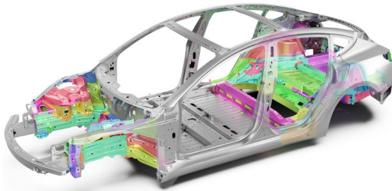
Model 3 body structure 171 pieces of metal highlighted
